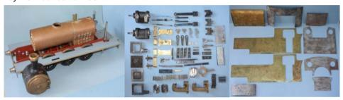
Part built 5 inch gauge 'Butch' 0-6-0. Professionally built silver soldered boiler by A W Thorne. Hydraulic tested and certified to 180psi. Most castings and plate work to complete the model are included. Full set of drawings by Kennion of Hertford £550
