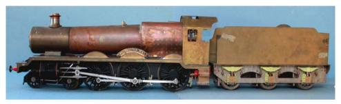
Part built 31/2 inch gauge GWR Hall Class. pump, brake linkage, silver soldered boiler. required to complete the model are included. Carry box. Full set of drawings by AJ Reeves. £1250
