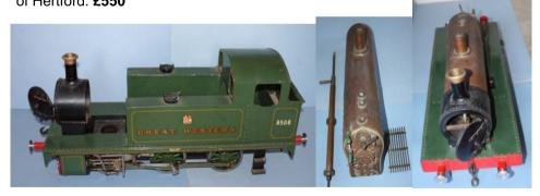
Part built 5 inch gauge Simplex 0-6-0. Copper silver soldered boiler, parts and castings, full set of drawings and 'Building Instructions' manual by Martin Evans. £1000
